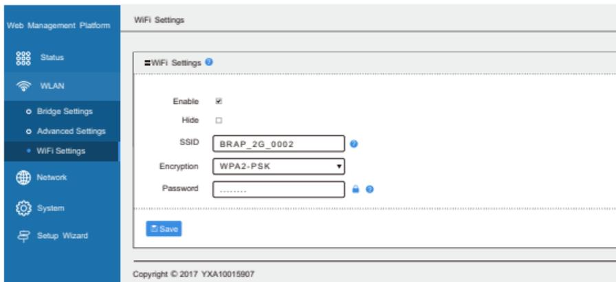
**Description:**The device launches the WiFi signal in the main AP mode.In the secondary AP mode, the WiFi signal is transmitted only after the bridge pairing is successfully connected.
